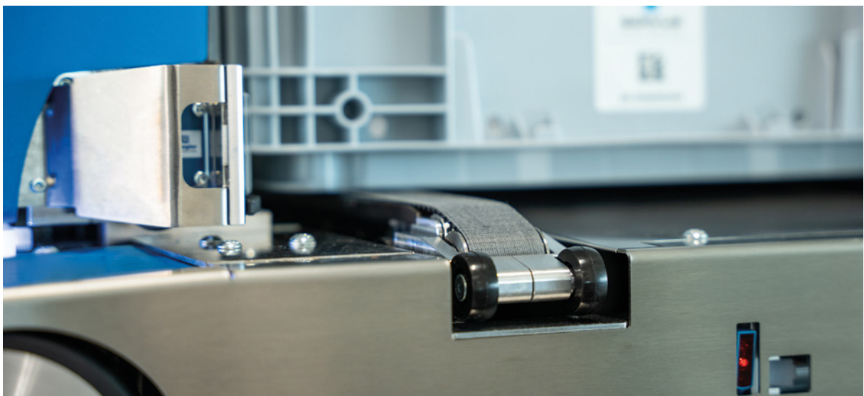
automatically adjusting side guide - © Servus Intralogistics
